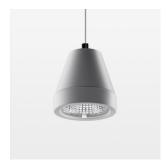
Suspended luminaire with LED, rated life of the LED L80/B10 > 50000 h, colour rendering index CRI > 80, chromaticity tolerance 3 SDCM (initial), rotation-symmetrical reflector with circular light distribution pattern, reflector pure aluminium 99,99% in MIRO-Silver®, segmented and faceted, 3D lens silicon to reduce the proportion of scattered light, luminaire head die-cast aluminium, powder-coated, stratosilver
