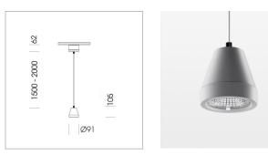
Suspended luminaire with LED, rated life of the LED L80/B10 > 50000 h, colour rendering index CRI > 80, chromaticity tolerance 3 SDCM (initial), rotation-symmetrical reflector with circular light distribution pattern, reflector pure aluminium 99,99% in MIRO-Silver®,segmented and faceted, 3D lens silicon to reduce the proportion of scattered light, luminaire head die-cast aluminium, powder-coated, stratosilver
