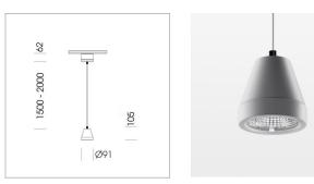
Suspended luminaire with LED, rated life of the LED L80/B10 > 50000 h, colour rendering index CRI > 90, chromaticity tolerance 3 SDCM (initial), rotation-symmetrical reflector with circular light distribution pattern, reflector pure aluminium 99,99% in MIRO-Silver®,segmented and faceted, 3D lens silicon to reduce the proportion of scattered light, luminaire head die-cast aluminium, powder-coated, stratosilver
