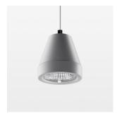
Suspended luminaire with LED, rated life of the LED L80/B10 > 50000 h, colour rendering index CRI > 95, chromaticity tolerance 2 SDCM (initial), rotation-symmetrical reflector with circular light distribution pattern, reflector pure aluminium 99,99% in MIRO-Silver®, segmented and faceted, 3D lens silicon to reduce the proportion of scattered light, luminaire head die-cast aluminium, powder-coated, stratosilver
