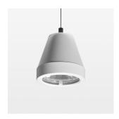
Suspended luminaire with LED, rated life of the LED L80/B10 > 50000 h, colour rendering index CRI > 95, chromaticity tolerance 2 SDCM (initial), rotation-symmetrical reflector with circular light distribution pattern, reflector pure aluminium 99,99% in MIRO-Silver®, segmented and faceted, 3D lens silicon to reduce the proportion of scattered light, luminaire head die-cast aluminium, powder-coated, stratowhite
