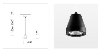
Suspended luminaire with LED, rated life of the LED L80/B10 > 50000 h, colour rendering index CRI > 90, chromaticity tolerance 2 SDCM (initial), rotation-symmetrical reflector with circular light distribution pattern, reflector pure aluminium 99,99% in MIRO-Silver®,segmented and faceted, 3D lens silicon to reduce the proportion of scattered light, luminaire head die-cast aluminium, powder-coated, stratoblack
