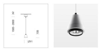
Suspended luminaire with LED, rated life of the LED L80/B10 > 50000 h, colour rendering index CRI > 80, chromaticity tolerance 2 SDCM (initial), reflector with circular light distribution pattern, reflector pure aluminium 99,99% in MIRO-Silver®,segmented and faceted, 3D lens silicon to reduce the proportion of scattered light, luminaire head die-cast aluminium, powdercoated, stratowhite
