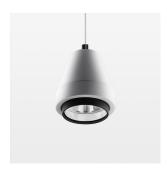
Suspended luminaire with LED, rated life of the LED L80/B10 > 50000 h, chromaticity tolerance 2 SDCM (initial), reflector with circular light distribution pattern, reflector pure aluminium 99,99% in MIRO-Silver®, segmented and faceted, 3D lens silicon to reduce the proportion of scattered light, luminaire head die-cast aluminium, powder-coated, stratowhite
