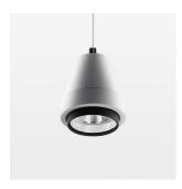
Suspended luminaire with LED, rated life of the LED L80/B10 > 50000 h, colour rendering index CRI > 90, chromaticity tolerance 2 SDCM (initial), reflector with circular light distribution pattern, reflector pure aluminium 99,99% in MIRO-Silver®, segmented and faceted, 3D lens silicon to reduce the proportion of scattered light, luminaire head die-cast aluminium, powder-coated, stratowhite
