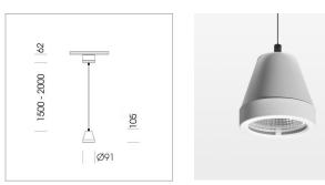
Suspended luminaire with LED, rated life of the LED L80/B10 > 50000 h, chromaticity tolerance 2 SDCM (initial), reflector with circular light distribution pattern, reflector pure aluminium 99,99% in MIRO-Silver®,segmented and faceted, 3D lens silicon to reduce the proportion of scattered light, luminaire head die-cast aluminium, powder-coated, stratowhite
