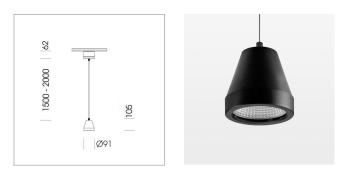
Suspended luminaire with LED, rated life of the LED L80/B10 > 50000 h, colour rendering index CRI > 90, chromaticity tolerance 2 SDCM (initial), reflector with circular light distribution pattern, reflector pure aluminium 99,99% in MIRO-Silver®,segmented and faceted, 3D lens silicon to reduce the proportion of scattered light, luminaire head die-cast aluminium, powdercoated, stratoblack
