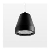
Suspended luminaire with LED, rated life of the LED L80/B10 > 50000 h, colour rendering index CRI > 96, chromaticity tolerance 3 SDCM (initial), reflector with circular light distribution pattern, reflector pure aluminium 99,99% in MIRO-Silver®, segmented and faceted, 3D lens silicon to reduce the proportion of scattered light, luminaire head die-cast aluminium, powder-coated, stratoblack
