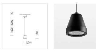
Suspended luminaire with LED, rated life of the LED L80/B10 > 50000 h, colour rendering index CRI > 80, chromaticity tolerance 2 SDCM (initial), reflector with circular light distribution pattern, reflector pure aluminium 99,99% in MIRO-Silver®,segmented and faceted, luminaire head die-cast aluminium, powder-coated, stratoblack
