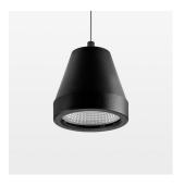
Suspended luminaire with LED, rated life of the LED L80/B10 > 50000 h, colour rendering index CRI > 90, chromaticity tolerance 2 SDCM (initial), reflector with circular light distribution pattern, reflector pure aluminium 99,99% in MIRO-Silver®, segmented and faceted, luminaire head die-cast aluminium, powder-coated, stratoblack
