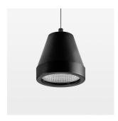
Suspended luminaire with LED, rated life of the LED L80/B10 > 50000 h, chromaticity tolerance 2 SDCM (initial), reflector with circular light distribution pattern, reflector pure aluminium 99,99% in MIRO-Silver®, segmented and faceted, luminaire head die-cast aluminium, powdercoated, stratoblack
