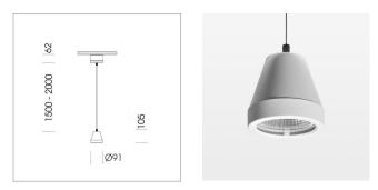
Suspended luminaire with LED, rated life of the LED L80/B10 > 50000 h, colour rendering index CRI > 90, chromaticity tolerance 2 SDCM (initial), reflector with circular light distribution pattern, reflector pure aluminium 99,99% in MIRO-Silver®,segmented and faceted, luminaire head die-cast aluminium, powder-coated, stratowhite
