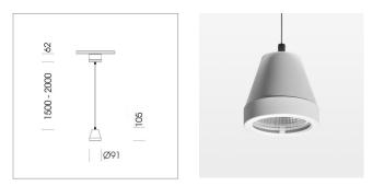
Suspended luminaire with LED, rated life of the LED L80/B10 > 50000 h, colour rendering index CRI > 96, chromaticity tolerance 3 SDCM (initial), reflector with circular light distribution pattern, reflector pure aluminium 99,99% in MIRO-Silver®,segmented and faceted, luminaire head die-cast aluminium, powder-coated, stratowhite
