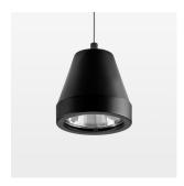
Suspended luminaire with LED, rated life of the LED L80/B10 > 50000 h, colour rendering index CRI > 80, chromaticity tolerance 3 SDCM (initial), rotation-symmetrical reflector with circular light distribution pattern, reflector pure aluminium 99,99% in MIRO-Silver®, segmented and faceted, 3D lens silicon to reduce the proportion of scattered light, luminaire head die-cast aluminium, powder-coated, stratoblack, separate driver unit
