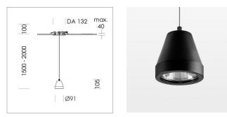
Suspended luminaire with LED, rated life of the LED L80/B10 > 50000 h, colour rendering index CRI > 96, chromaticity tolerance 2 SDCM (initial), rotation-symmetrical reflector with circular light distribution pattern, reflector pure aluminium 99,99% in MIRO-Silver®,segmented and faceted, 3D lens silicon to reduce the proportion of scattered light, luminaire head die-cast aluminium, powder-coated, stratoblack, separate driver unit
