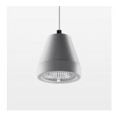
Suspended luminaire with LED, rated life of the LED L80/B10 > 50000 h, colour rendering index CRI > 80, chromaticity tolerance 3 SDCM (initial), rotation-symmetrical reflector with circular light distribution pattern, reflector pure aluminium 99,99% in MIRO-Silver®, segmented and faceted, 3D lens silicon to reduce the proportion of scattered light, luminaire head die-cast aluminium, powder-coated, stratosilver, separate driver unit
