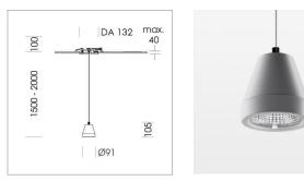
Suspended luminaire with LED, rated life of the LED L80/B10 > 50000 h, colour rendering index CRI > 80, chromaticity tolerance 3 SDCM (initial), rotation-symmetrical reflector with circular light distribution pattern, reflector pure aluminium 99,99% in MIRO-Silver®,segmented and faceted, 3D lens silicon to reduce the proportion of scattered light, luminaire head die-cast aluminium, powder-coated, stratosilver, separate driver unit
