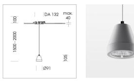
Suspended luminaire with LED, rated life of the LED L80/B10 > 50000 h, colour rendering index CRI > 90, chromaticity tolerance 3 SDCM (initial), rotation-symmetrical reflector with circular light distribution pattern, reflector pure aluminium 99,99% in MIRO-Silver®,segmented and faceted, 3D lens silicon to reduce the proportion of scattered light, luminaire head die-cast aluminium, powder-coated, stratosilver, separate driver unit
