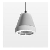
Suspended luminaire with LED, rated life of the LED L80/B10 > 50000 h, colour rendering index CRI > 95, chromaticity tolerance 2 SDCM (initial), rotation-symmetrical reflector with circular light distribution pattern, reflector pure aluminium 99,99% in MIRO-Silver®, segmented and faceted, 3D lens silicon to reduce the proportion of scattered light, luminaire head die-cast aluminium, powder-coated, stratowhite, separate driver unit
