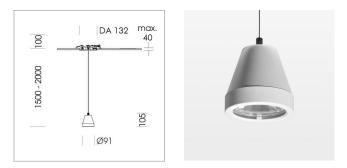
Suspended luminaire with LED, rated life of the LED L80/B10 > 50000 h, colour rendering index CRI > 96, chromaticity tolerance 2 SDCM (initial), rotation-symmetrical reflector with circular light distribution pattern, reflector pure aluminium 99,99% in MIRO-Silver®,segmented and faceted, 3D lens silicon to reduce the proportion of scattered light, luminaire head die-cast aluminium, powder-coated, stratowhite, separate driver unit
