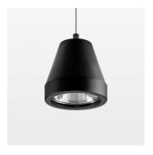
Suspended luminaire with LED, rated life of the LED L80/B10 > 50000 h, colour rendering index CRI > 90, chromaticity tolerance 2 SDCM (initial), rotation-symmetrical reflector with circular light distribution pattern, reflector pure aluminium 99,99% in MIRO-Silver®, segmented and faceted, 3D lens silicon to reduce the proportion of scattered light, luminaire head die-cast aluminium, powder-coated, stratoblack, separate driver unit
