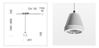
Suspended luminaire with LED, rated life of the LED L80/B10 > 50000 h, colour rendering index CRI > 90, chromaticity tolerance 2 SDCM (initial), rotation-symmetrical reflector with circular light distribution pattern, reflector pure aluminium 99,99% in MIRO-Silver®,segmented and faceted, 3D lens silicon to reduce the proportion of scattered light, luminaire head die-cast aluminium, powder-coated, stratowhite, separate driver unit
