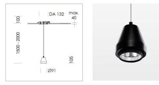
Suspended luminaire with LED, rated life of the LED L80/B10 > 50000 h, chromaticity tolerance 2 SDCM (initial), reflector with circular light distribution pattern, reflector pure aluminium 99,99% in MIRO-Silver®,segmented and faceted, 3D lens silicon to reduce the proportion of scattered light, luminaire head die-cast aluminium, powder-coated, stratoblack, separate driver unit
