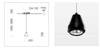
Suspended luminaire with LED, rated life of the LED L80/B10 > 50000 h, colour rendering index CRI > 96, chromaticity tolerance 3 SDCM (initial), reflector with circular light distribution pattern, reflector pure aluminium 99,99% in MIRO-Silver®,segmented and faceted, 3D lens silicon to reduce the proportion of scattered light, luminaire head die-cast aluminium, powdercoated, stratoblack, separate driver unit
