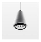
Suspended luminaire with LED, rated life of the LED L80/B10 > 50000 h, colour rendering index CRI > 80, chromaticity tolerance 2 SDCM (initial), reflector with circular light distribution pattern, reflector pure aluminium 99,99% in MIRO-Silver®, segmented and faceted, 3D lens silicon to reduce the proportion of scattered light, luminaire head die-cast aluminium, powder-coated, stratowhite, separate driver unit
