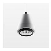
Suspended luminaire with LED, rated life of the LED L80/B10 > 50000 h, colour rendering index CRI > 90, chromaticity tolerance 2 SDCM (initial), reflector with circular light distribution pattern, reflector pure aluminium 99,99% in MIRO-Silver®, segmented and faceted, 3D lens silicon to reduce the proportion of scattered light, luminaire head die-cast aluminium, powder-coated, stratowhite, separate driver unit
