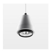
Suspended luminaire with LED, rated life of the LED L80/B10 > 50000 h, chromaticity tolerance 2 SDCM (initial), reflector with circular light distribution pattern, reflector pure aluminium 99,99% in MIRO-Silver®, segmented and faceted, 3D lens silicon to reduce the proportion of scattered light, luminaire head die-cast aluminium, powder-coated, stratowhite, separate driver unit
