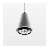
Suspended luminaire with LED, rated life of the LED L80/B10 > 50000 h, colour rendering index CRI > 96, chromaticity tolerance 3 SDCM (initial), reflector with circular light distribution pattern, reflector pure aluminium 99,99% in MIRO-Silver®, segmented and faceted, 3D lens silicon to reduce the proportion of scattered light, luminaire head die-cast aluminium, powder-coated, stratowhite, separate driver unit
