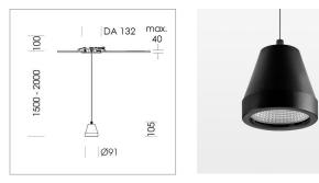
Suspended luminaire with LED, rated life of the LED L80/B10 > 50000 h, chromaticity tolerance 2 SDCM (initial), reflector with circular light distribution pattern, reflector pure aluminium 99,99% in MIRO-Silver®,segmented and faceted, 3D lens silicon to reduce the proportion of scattered light, luminaire head die-cast aluminium, powder-coated, stratoblack, separate driver unit
