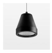
Suspended luminaire with LED, rated life of the LED L80/B10 > 50000 h, chromaticity tolerance 2 SDCM (initial), reflector with circular light distribution pattern, reflector pure aluminium 99,99% in MIRO-Silver®, segmented and faceted, 3D lens silicon to reduce the proportion of scattered light, luminaire head die-cast aluminium, powder-coated, stratoblack, separate driver unit
