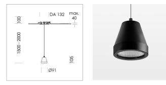
Suspended luminaire with LED, rated life of the LED L80/B10 > 50000 h, colour rendering index CRI > 90, chromaticity tolerance 2 SDCM (initial), reflector with circular light distribution pattern, reflector pure aluminium 99,99% in MIRO-Silver®,segmented and faceted, 3D lens silicon to reduce the proportion of scattered light, luminaire head die-cast aluminium, powdercoated, stratoblack, separate driver unit
