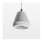
Suspended luminaire with LED, rated life of the LED L80/B10 > 50000 h, chromaticity tolerance 2 SDCM (initial), reflector with circular light distribution pattern, reflector pure aluminium 99,99% in MIRO-Silver®, segmented and faceted, 3D lens silicon to reduce the proportion of scattered light, luminaire head die-cast aluminium, powder-coated, stratowhite, separate driver unit
