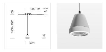
Suspended luminaire with LED, rated life of the LED L80/B10 > 50000 h, chromaticity tolerance 2 SDCM (initial), reflector with circular light distribution pattern, reflector pure aluminium 99,99% in MIRO-Silver®,segmented and faceted, 3D lens silicon to reduce the proportion of scattered light, luminaire head die-cast aluminium, powder-coated, stratowhite, separate driver unit
