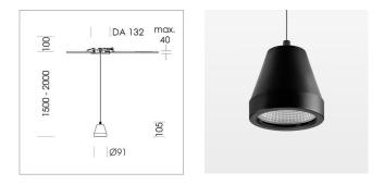
Suspended luminaire with LED, rated life of the LED L80/B10 > 50000 h, colour rendering index CRI > 80, chromaticity tolerance 2 SDCM (initial), reflector with circular light distribution pattern, reflector pure aluminium 99,99% in MIRO-Silver®,segmented and faceted, luminaire head die-cast aluminium, powder-coated, stratoblack, separate driver unit
