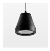
Suspended luminaire with LED, rated life of the LED L80/B10 > 50000 h, colour rendering index CRI > 80, chromaticity tolerance 2 SDCM (initial), reflector with circular light distribution pattern, reflector pure aluminium 99,99% in MIRO-Silver®, segmented and faceted, luminaire head die-cast aluminium, powder-coated, stratoblack, separate driver unit
