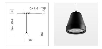
Suspended luminaire with LED, rated life of the LED L80/B10 > 50000 h, colour rendering index CRI > 96, chromaticity tolerance 3 SDCM (initial), reflector with circular light distribution pattern, reflector pure aluminium 99,99% in MIRO-Silver®,segmented and faceted, luminaire head die-cast aluminium, powder-coated, stratoblack, separate driver unit
