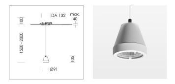
Suspended luminaire with LED, rated life of the LED L80/B10 > 50000 h, colour rendering index CRI > 80, chromaticity tolerance 2 SDCM (initial), reflector with circular light distribution pattern, reflector pure aluminium 99,99% in MIRO-Silver®,segmented and faceted, luminaire head die-cast aluminium, powder-coated, stratowhite, separate driver unit
