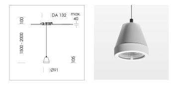
Suspended luminaire with LED, rated life of the LED L80/B10 > 50000 h, colour rendering index CRI > 90, chromaticity tolerance 2 SDCM (initial), reflector with circular light distribution pattern, reflector pure aluminium 99,99% in MIRO-Silver®,segmented and faceted, luminaire head die-cast aluminium, powder-coated, stratowhite, separate driver unit
