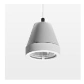
Suspended luminaire with LED, rated life of the LED L80/B10 > 50000 h, chromaticity tolerance 2 SDCM (initial), reflector with circular light distribution pattern, reflector pure aluminium 99,99% in MIRO-Silver®, segmented and faceted, luminaire head die-cast aluminium, powdercoated, stratowhite, separate driver unit
