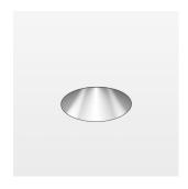
Recessed downlight, flush with ceiling with LED, rated life of the LED L80/B10 > 50000 h, colour rendering index CRI > 80, chromaticity tolerance 2 SDCM (initial), reflector with homogeneous light distribution pattern, diffuser lens, translucent, darklight reflector, aluminium, metallised, highgloss, luminaire head die-cast aluminium, black anodized black anodized, Ceiling plaster die-cast aluminum, trim plastic injection molding, black, separate driver unit
