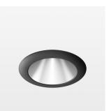
Recessed downlight with LED, rated life of the LED L80/B10 > 50000 h, colour rendering index CRI > 96, chromaticity tolerance 2 SDCM (initial), reflector with homogeneous light distribution pattern, diffuser lens, translucent, darklight reflector, aluminium, metallised, highgloss, luminaire head die-cast aluminium, powder-coated, mounting ring die-cast aluminum, front ring and coverblind plastic, black, separate driver unit
