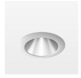
Recessed downlight with LED, rated life of the LED L80/B10 > 50000 h, colour rendering index CRI > 96, chromaticity tolerance 2 SDCM (initial), reflector with homogeneous light distribution pattern, diffuser lens, translucent, darklight reflector, aluminium, metallised, highgloss, luminaire head die-cast aluminium, powder-coated, mounting ring die-cast aluminum, front ring and coverblind plastic, white, separate driver unit
