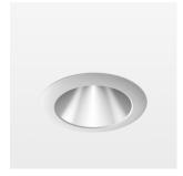
Recessed downlight with LED, rated life of the LED L80/B10 > 500000 h, colour rendering index CRI > 96, chromaticity tolerance 2 SDCM (initial), reflector with homogeneous light distribution pattern, diffuser lens, translucent, darklight reflector, aluminium, metallised, highgloss, luminaire head die-cast aluminium, powder-coated, mounting ring die-cast aluminum, front ring and coverblind plastic, white, separate driver unit
