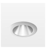
Recessed downlight with LED, rated life of the LED L80/B10 > 50000 h, chromaticity tolerance 3 SDCM (initial), reflector with homogeneous light distribution pattern, diffuser lens, translucent, darklight reflector, aluminium, metallised, highgloss, luminaire head die-cast aluminium, powder-coated, mounting ring die-cast aluminum, front ring and coverblind plastic, white, separate driver unit
