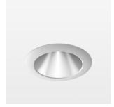
Recessed downlight with LED, rated life of the LED L80/B10 > 50000 h, chromaticity tolerance 3 SDCM (initial), reflector with homogeneous light distribution pattern, diffuser lens, translucent, darklight reflector, aluminium, metallised, highgloss, luminaire head die-cast aluminium, powder-coated, mounting ring die-cast aluminum, front ring and coverblind plastic, white, separate driver unit
