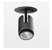
Semi-recessed luminaire with LED, rated life of the LED L80/B10 > 50000 h, chromaticity tolerance 2 SDCM (initial), , reflector with circular light distribution pattern, reflector pure aluminium 99,99% in MIRO-Silver®, segmented and faceted, exchangeable reflector unit in high-sheen black plastic, with glass cover, luminaire head die-cast aluminium, powder-coated, rotation angle 330°, swivel angle +90°/-90°, luminaire housing die-cast aluminium, powder-coated, stratoblack, separate driver unit
